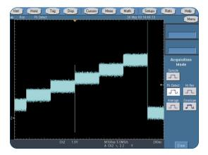
Peak detect mode enables the TDS7000 Series oscilloscope to capture transient anomalies as narrow as 100 ps.
