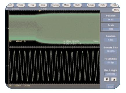
Capturing the high frequency detail of this modulated 85 MHz carrier requires high resolution sampling (100 ps). Seeing the signal's complete modulation envelope requires a long time duration (1 ms). Using long record length (10 MB), the oscilloscope can display both.
