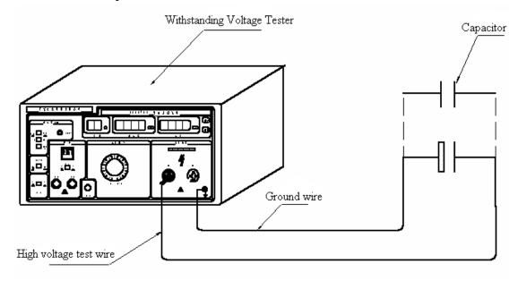
a) Judgment of high voltage silicon stack and high-voltage power transistor's  $BV_{\text{CEO.}}$
