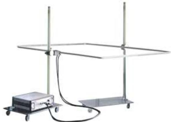
The increased antenna size means that objects up of 1.2m x 1.6m can be tested. However, because the coil antenna is still used with the MAG 100 current transformer, maximum current in the coil is 120A. This results in a magnetic field of only 36A/m at coil center.
