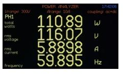
Using the zoom key any four selected measurement items can be enlarged even further for easy viewing.
