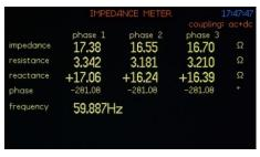
Utilising true real time DFT analysis, the PPA1500 provides precision impedance measurements on any individual phase or a simultaneous display of all three phases as shown here.
