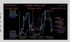
Datalog periods can be set with no gap so that no information is missed during datalog capture and the display is updated during datalog with real time, tabular or graphic display.
