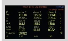
In addition to the true rms value of voltage and current on any measurement channel, **RMS** mode also provides real time analysis of dc, ac, peak, factor, surge, mean and form factor.
